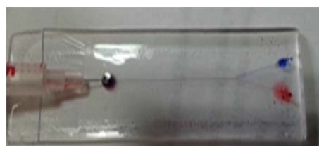
(b) Mixing behavior of Y micro-mixer after filling with colors
