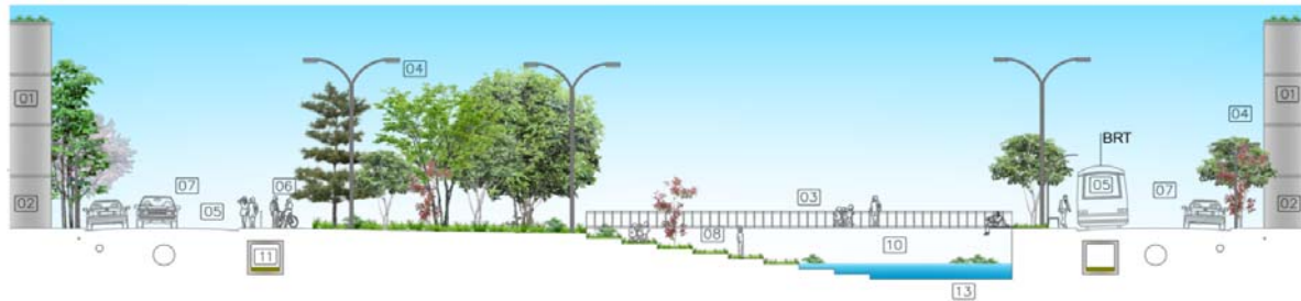
Fig. 5 Typical cut for the proposed blue and green corridors. Source: Prepared by the authors. (1) Multiple use buildings with green roof; (2) Living Ground Floor with commercial units; (3) Crossing bridge for pedestrians; (4) Planting of suitable species; (5) Public transportation; (6) Bike trail; (7) Limitation of the use of individual transport; (8) Roof terrace; (9) Sustainable drainage; (10) Use of phytoremediation species in the watercourse; (11) Sustainable drainage; (12) Health infrastructure; (13) Regularization of the canal bed with sustainable techniques; (14) Adequate lighting to promote nighttime use of structures
