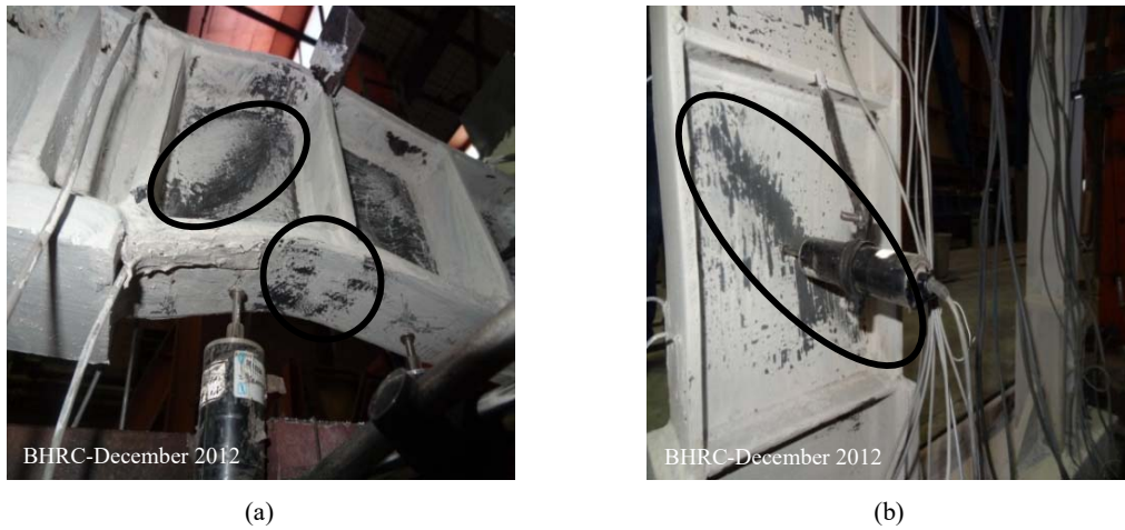
Fig. 5 Uniform shear yielding and diagonal tension field (30th cycle) formation in web of: (a) H.P.G, (b) V.P.G
