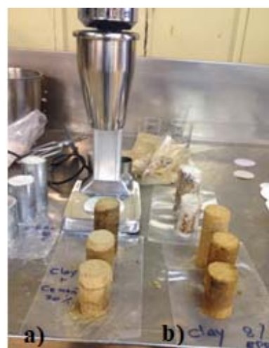
Fig. 2 Soil A with cement (a), with epoxy (b)
