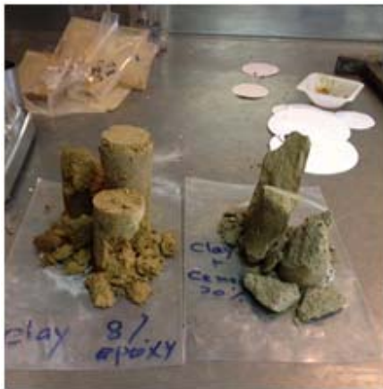
Fig. 4 Soil specimens after compression tests
