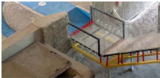
Fig. 1 Hydraulic model of Nazloochoy dam
