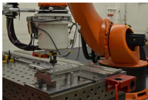
Fig. 4 Robotized FSW setup for stationary shoulder and conventional FSW
