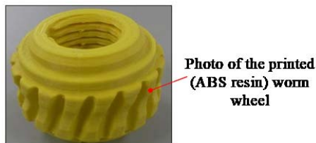
Fig. 11 Design process of the worm wheel, showing a photo of the printed wheel in ABS resin
