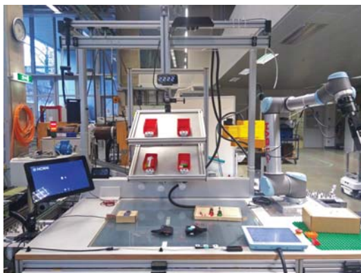
Fig. 4 The assembly table equipped with a tablet-PC, a projector, a screen below the working surface, light-indicators, sensors and a collaborative robot
