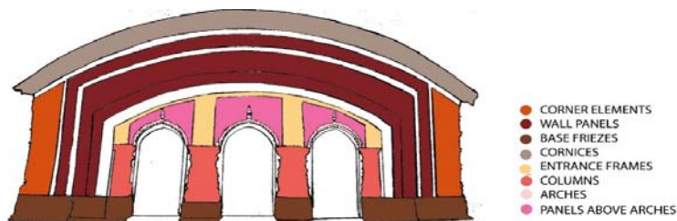
Fig. 28 Schematic Triple-entrance Façades
