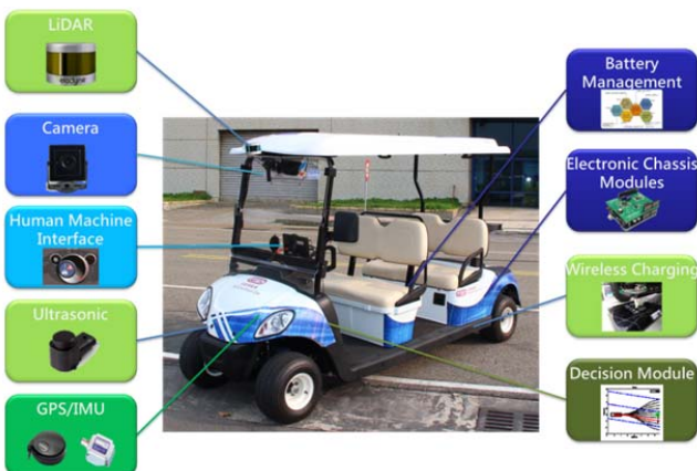
Fig. 8 The in-house built self-driving e-golf cart
