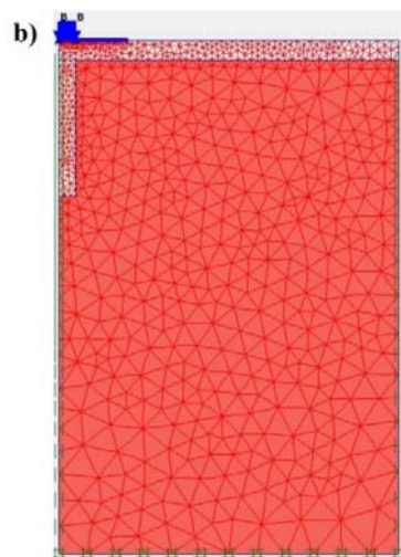
Fig. 3 Axisymmetrical numerical model in dynamic analysis, (a) Harmonic load on the surface, (b) mesh sizes in dynamic analysis
