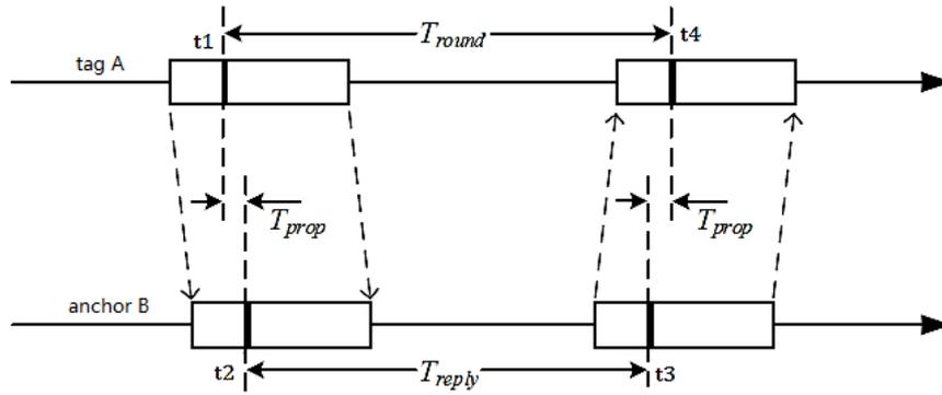
Fig. 1 Process of message passing in SS-TWR
