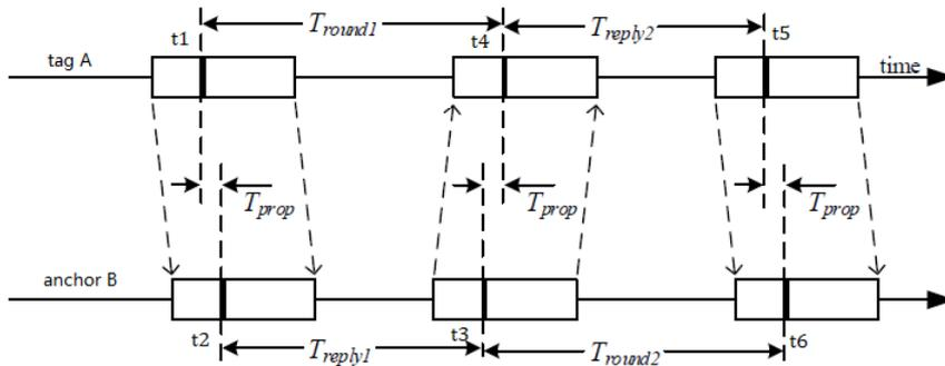
Fig. 2 Process of message passing in DS-TWR
