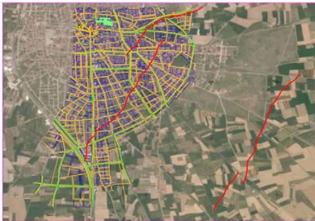
Fig. 2 The surface deformations which are parallel and semi-parallel to Bolvadin fault
