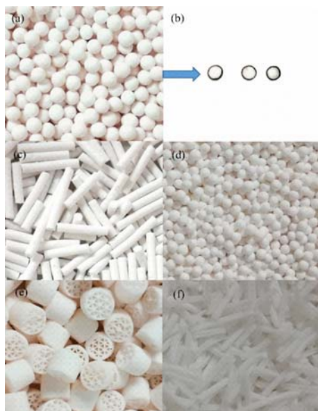
Fig. 1 Different shape of supports: (a) SiO 2 -Sphere (d=2.2 mm), (b) cross section of eggshell catalyst (Co/Nb-SiO 2 -Eggshell, d=2.2 mm, Δd=120~160 μm), (c) SiO 2 -Extrusion (d=2.0 mm), (d) Al 2 O 3 -Sphere (d=1.7 mm), (e) Al 2 O 3 -Wheel (d=5.0 mm), and (f) Al 2 O 3 -Trefoil (d=1.5 mm)
