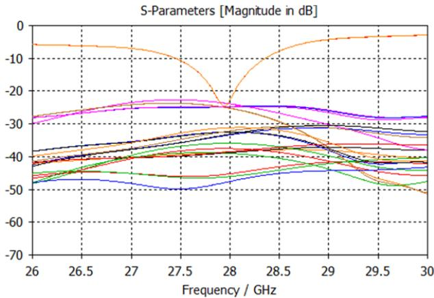
Fig. 7 Port isolations S11, S21, S31, etc.
