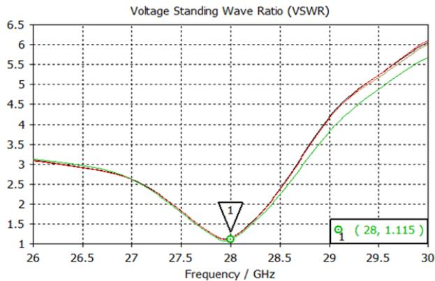
Fig. 10 Voltage Standing Wave Ratio array 8x2 antenna
