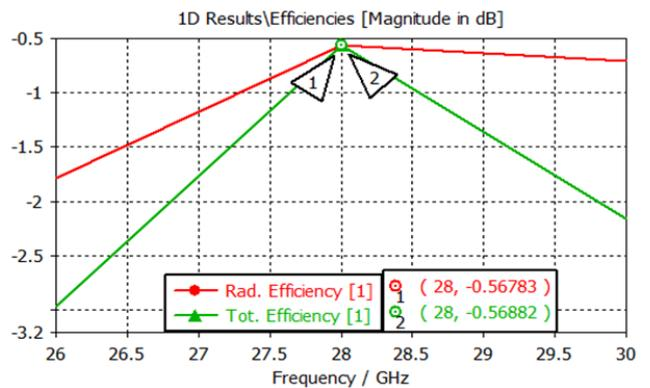
Fig. 5 Radiation and total efficiency of single antenna
