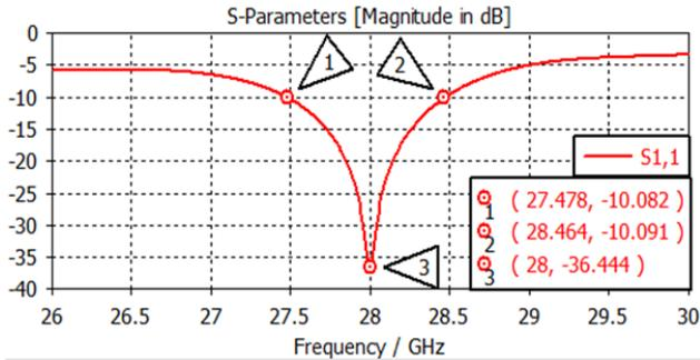
Fig. 2 Return loss of single element antenna
