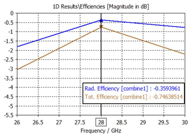
Fig. 9 Radiation and Total Efficiency of Array Antenna
