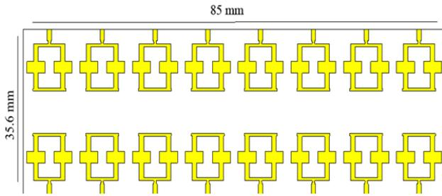
Fig. 6 Dimension of 8x2 linear array antenna
