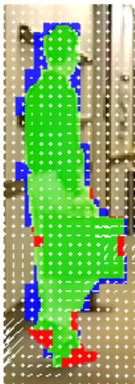
Fig. 5 Tracking result with PVM assignment. True positives (TPs) are shown as green, false positives (FPs) as blue and false negatives (FNs) as red
