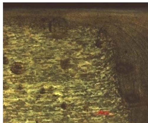
Fig. 7 (c) Microstructure of the THAZ zone in FSW weld
