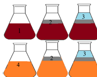
Fig. 2 Flask A (The Digesters). 1. Blood or RBCs. 2. Bacteria. 3. Water. 4. Blood platelet (BPL). Note: 1000 g = flask capacity, 100 g = bacteria weight
