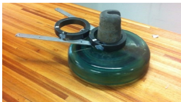
Fig. 10 Adapted prototype LC sensor with its mechanical clamps around a glass insulator
