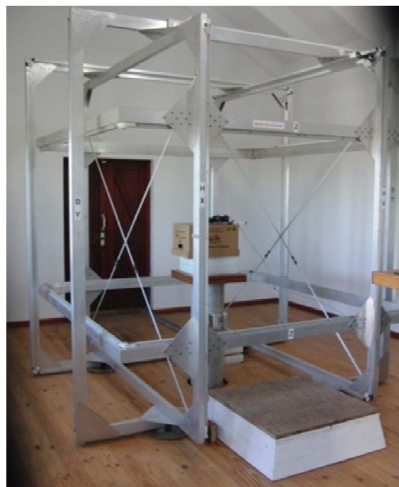
Fig. 11 3-axes Helmholtz coil system for calibration of the prototype LC sensor
