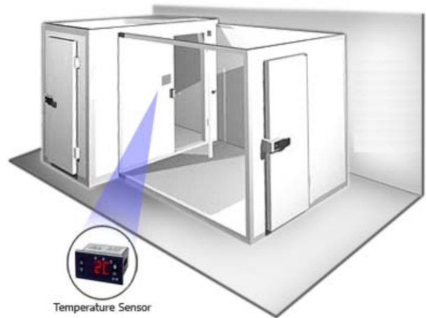
Fig. 5 Cold room for fruits refrigeration
