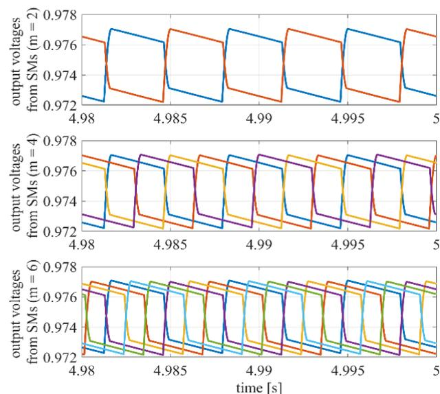
Fig. 4 Steady state SM voltages for different number of SMs
