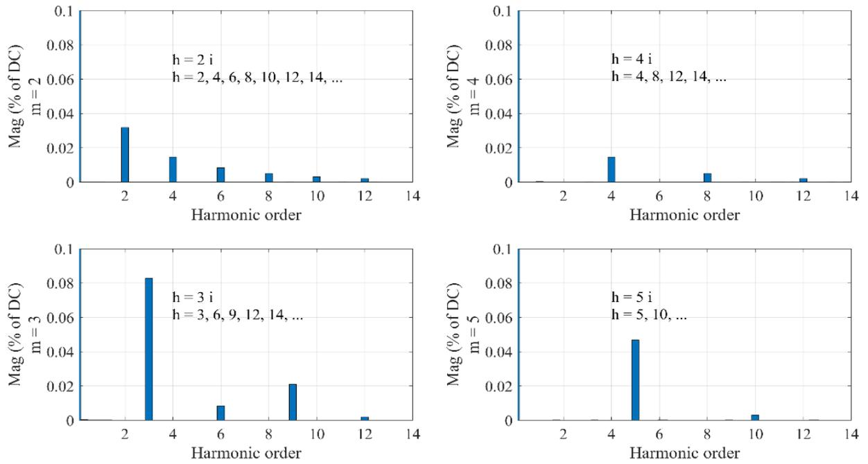
Fig. 6 FFT analysis of the generator output voltages ( $m = 2, 3, 4$  &  $5$ )
