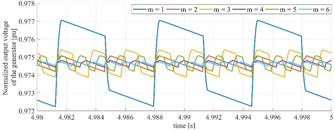
Fig. 5 Steady state normalized output voltages from the proposed generator for different number of SMs
