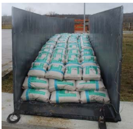
Fig. 15 Perform static loading test on footbridge I
