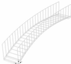
Fig. 3 Segmentation of macroelements to surfaces
