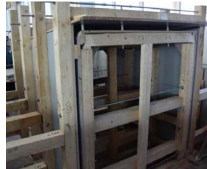
Fig. 8 Formwork of test sample
