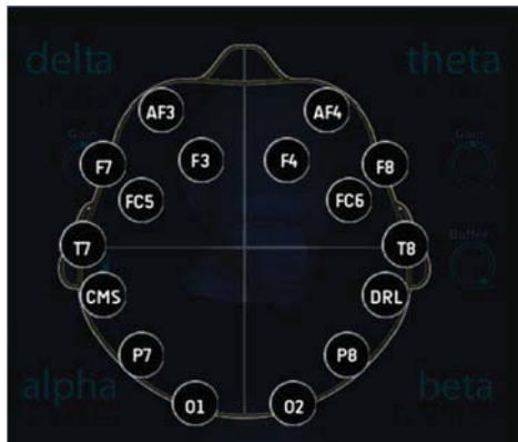
Fig. 5 Emotiv epoc+ EEG Sensors, 14 EEG sensors (AF3, F7, F3, FC5, T7, P7, O1, O2, P8, T8, FC6, F4, F8 and AF4), 2 references (CMS and DRL)
