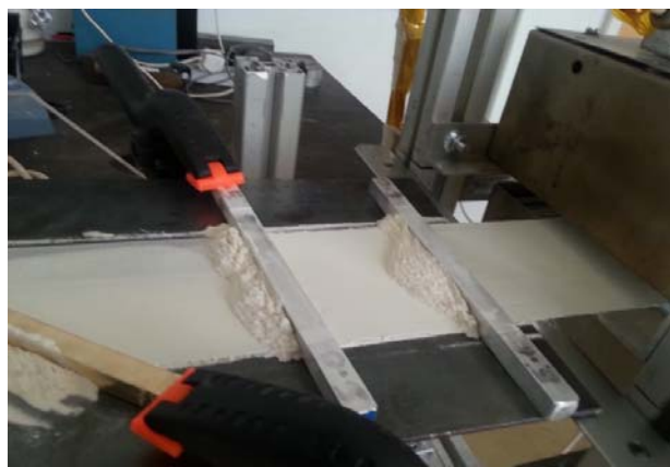
Fig. 2 Powder deposition setup
