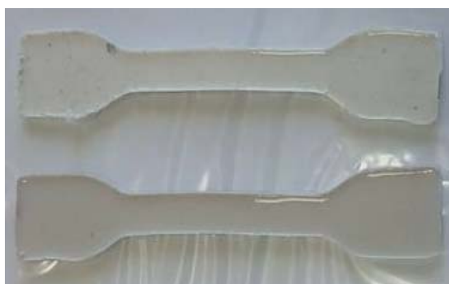
Fig. 6 Moulded Ag doped CNFs/RTV664 composite
