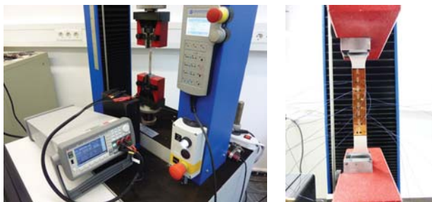
(a) Tensile test with reference strain gauge (b) Clamped tensile specimen with AJP strain gauges
