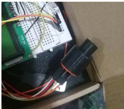
Fig. 3 Mouthpiece with MQ 138 sensor
