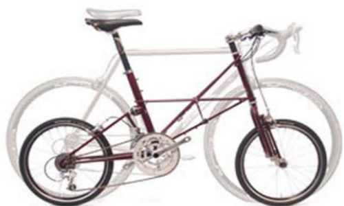
Fig. 1 Comparison between typical big wheel bicycle and Moulton small wheel bicycle
