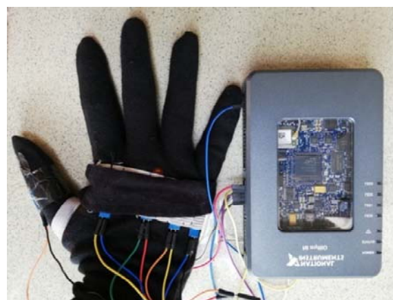
Fig. 2 Gesture digitization glove assembly
