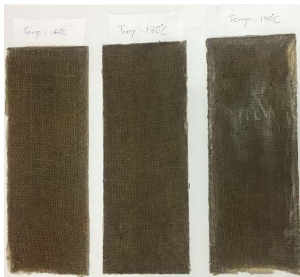
Fig. 3 Developed Jute/PLA composites at different curing temperature
