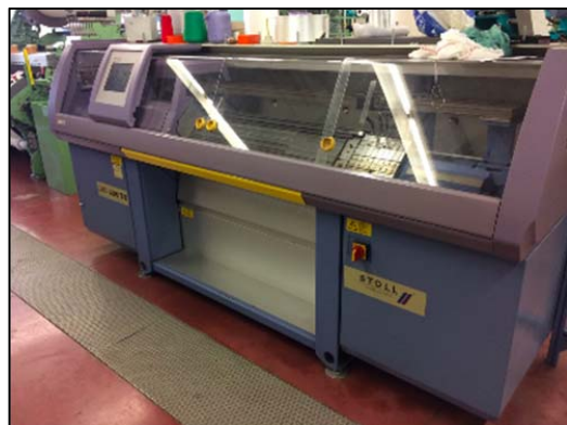
Fig. 1 Flat bed knitting machine used to produce plain knits and auxetic knitted fabrics
