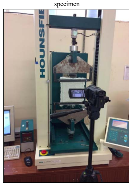
Fig. 6 Setup of testing Poisson's ratio
