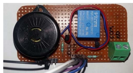
Fig. 2 Control circuit module
