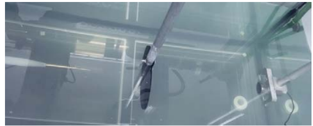
Fig. 3 Picture of the experimental set-up where hydrophone, FZP and piston transducer are shown
