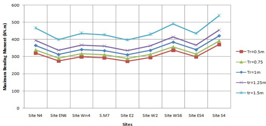
Fig. 9 Maximum moment at raft foundation for different foundation thickness and different sites
