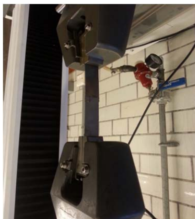
Fig. 5 Single-lab shear test setup
