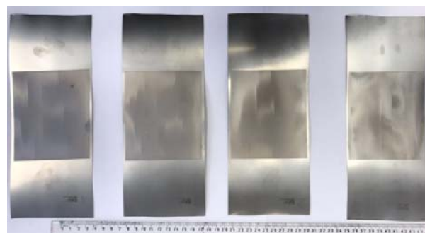
Fig.3 The effect of the parameter of the laser treatment on the surface roughness of titanium alloy
