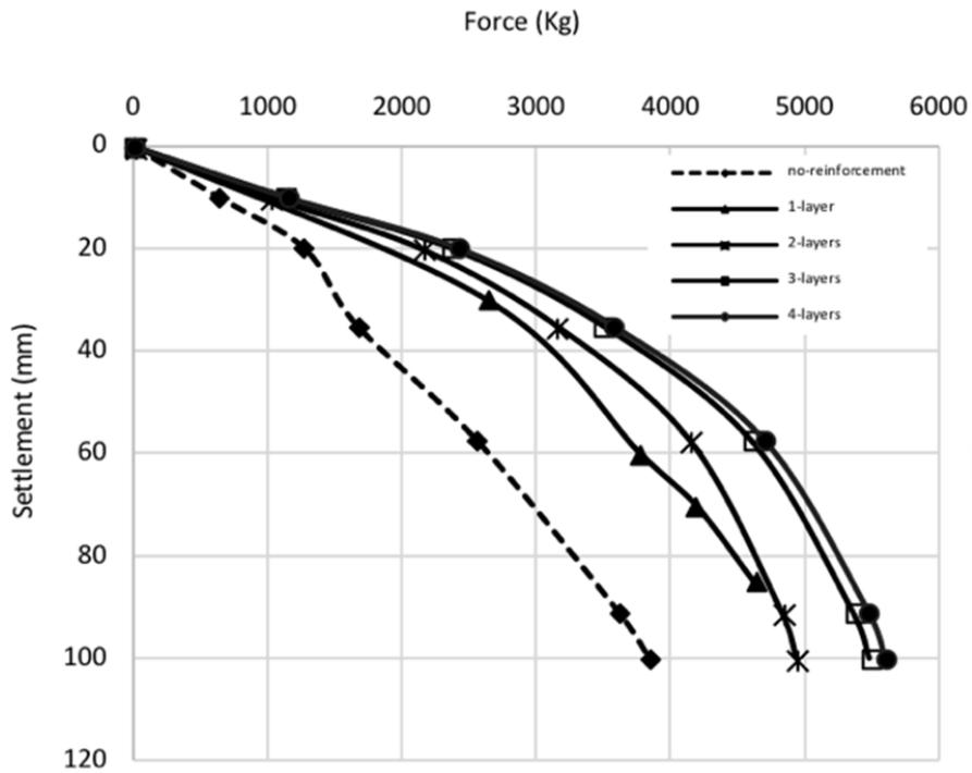
Fig. 2 The influence of number of geogrid layers on the bearing capacity obtained from the plate loading test in a double-layer soil with a top layer thickness (gravel) of 0.5B
