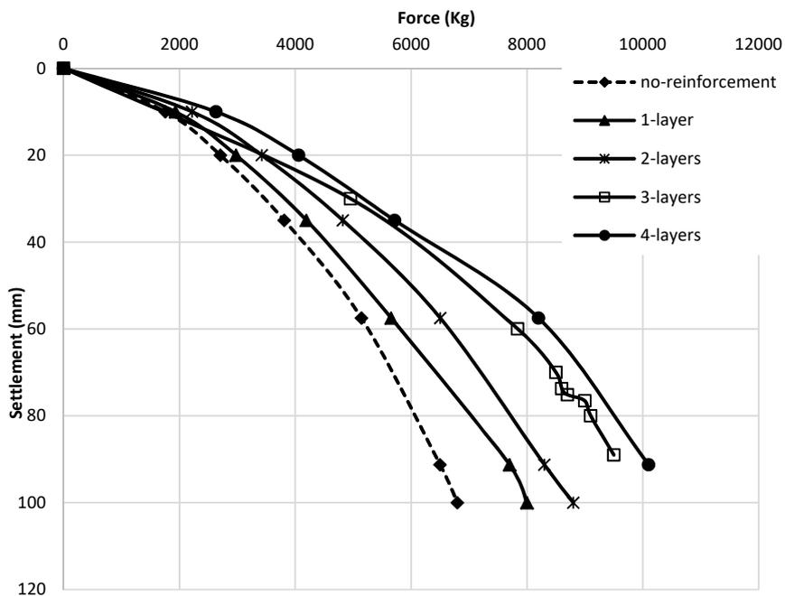
Fig. 5 The influence of number of geogrid layers on the bearing capacity obtained from the plate loading test in a double-layer soil with a top layer thickness (gravel) of 2.0B
