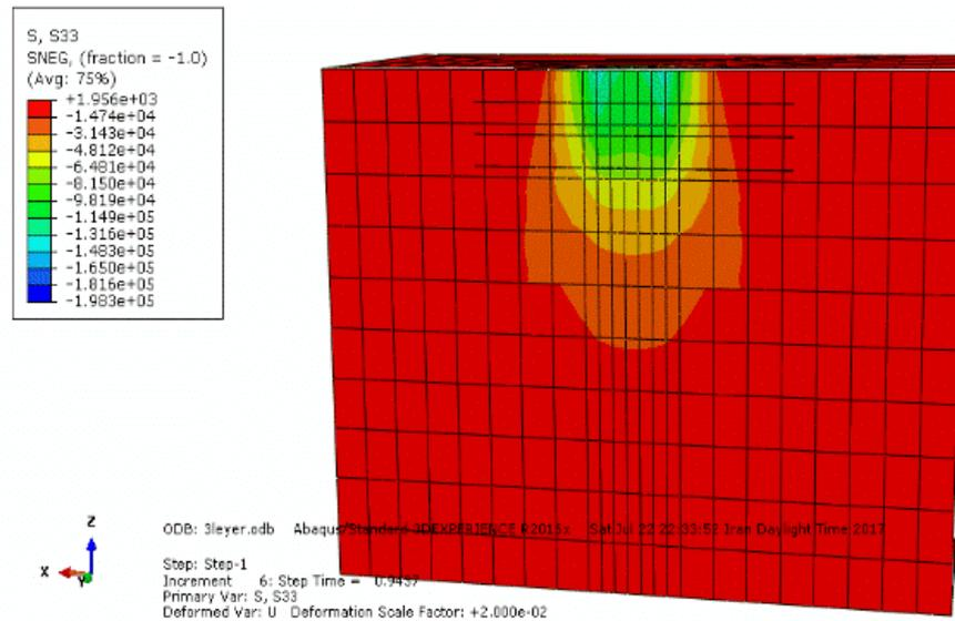
Fig. 9 The contour of vertical stress in a double-layer soil reinforced by three layers of geogrid with a top layer thickness (gravel) of 2.0B
