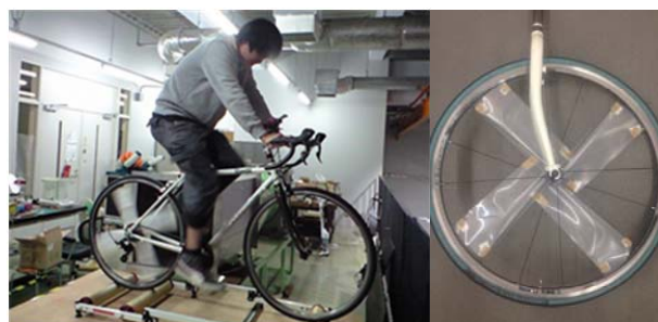
Fig. 1 Bicycle with Wells turbine in wheels
