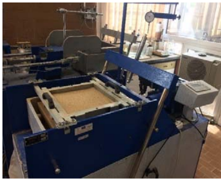
Fig. 3 Large scale direct shear tests on sandy soil in loose condition
