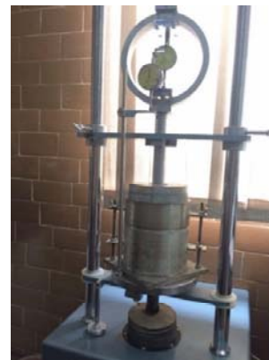
Fig. 6 CBR tests on sandy subgrade in loose condition
