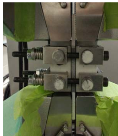
Fig. 3 Compression test using anti-buckling fixture, using the thickness side for measuring the strain by DIC
