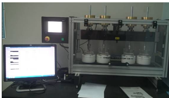
Fig. 3 Chewing simulator with the testing system's computer monitoring software
