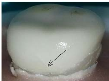
Fig. 6 Lingual surface of sample no. 1 of 0.5 mm group after mouth-motion fatigue testing indicating its crack pattern
