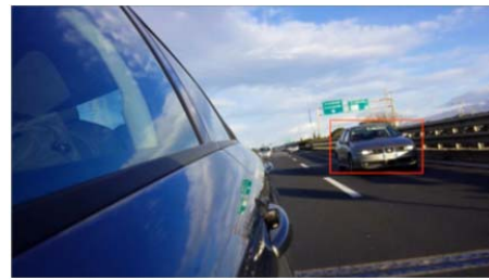
Fig. 6 Example of warning alert; the distance of the overtaking vehicle is lower than 5 m, so the bounding box is signed as red
