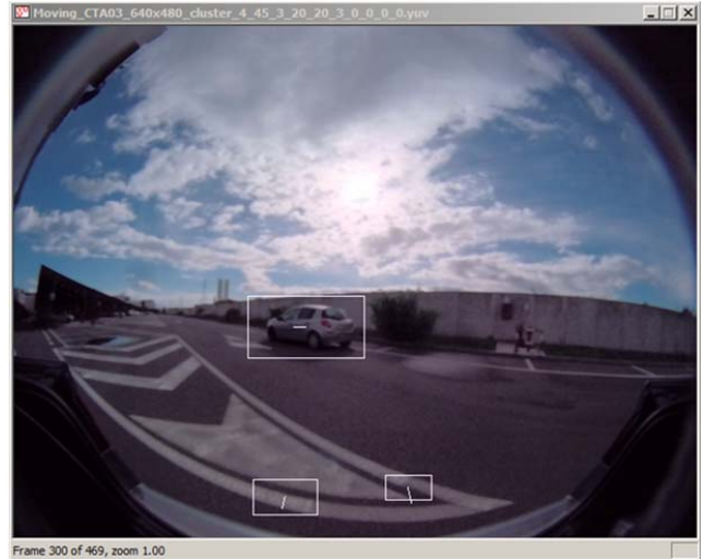
Fig. 8 Rear CTA example: Clustering output
