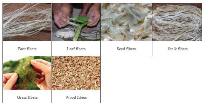
Fig. 1 Types of plant-based natural fibers from left to right: bast fibers, leaf fibers, seed fibers, stalk fibers, grass fibers and wood fibers
