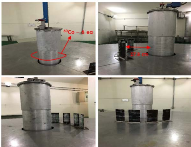
Fig. 2 Experimental set-up of gamma-ray irradiation of NPT-IGBTs
