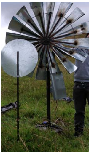
Fig. 6 Prototype built to perform performance tests
