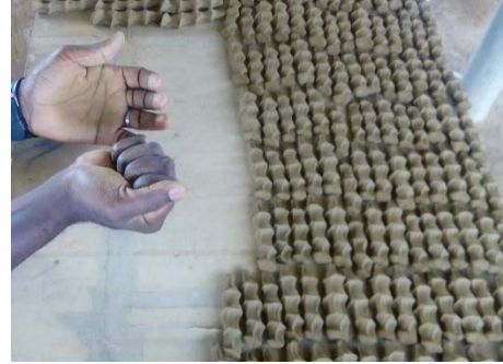
Fig. 5 Compressing the clay in the fist to transfer the imprint of the fingers onto it
