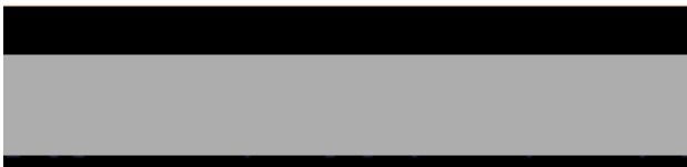
Fig. 4 Initial interface shape for multi-mode film boiling (black – vapor; gray – liquid)
