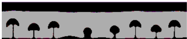
Fig. 6 Interface shape for multi-mode film boiling at 2 s (black – vapor; gray – liquid)
