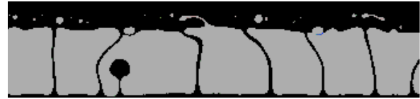
Fig. 8 Interface shape for multi-mode film boiling at 4s (black – vapor; gray – liquid)
