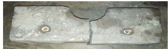
Fig. 7 Concrete block after flexural strength
