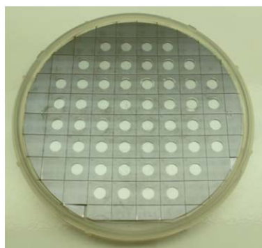
Fig. 5 Photo of the bonded wafer pair (4") after bonding and dicing, showing the absence of unbonded areas
