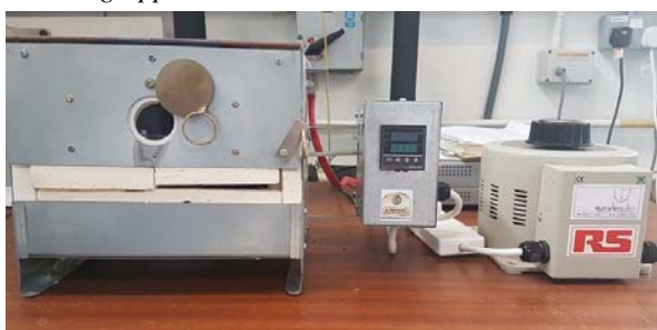
Fig. 3 Kiln with Transformer
